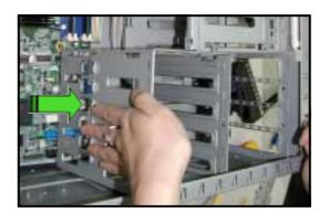
3. Make sure that the drive cage is fits snugly to the bay as shown. The drive cage is properly installed when it is parallel to the front panel, and the screw hole matches the hole of the first drive cage.
